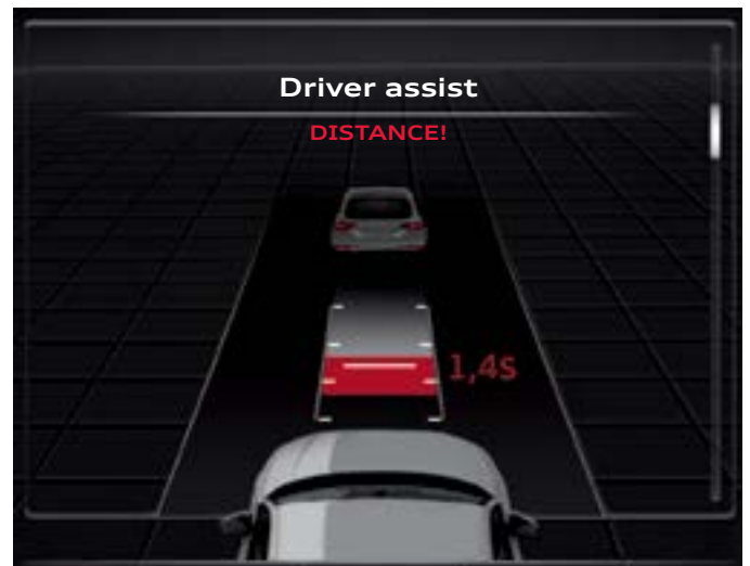
Distance warning if the distance to the preceding vehicle is less than the distance set by the driver
