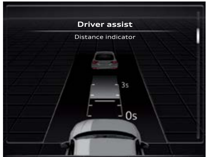
Distance indicator in case of vehicle in front
