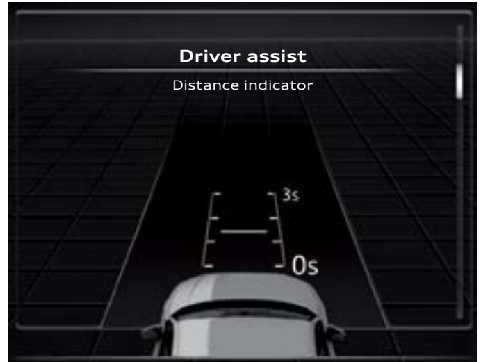
Distance indicator if no preceding vehicle is detected
