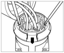
The kit includes detailed instructions for disconnecting, unlocking, disassembling and repairing most of the different types of multi-point connector currently in use in Audi vehicles. The illustrations shown here are examples.
