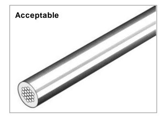
Inspect especially where a cable tie or other fastener has been used to secure the harness. If it has been installed too tightly, and the insulation has been damaged, it may be necessary to make the repair in a different place, where there is undamaged wire.
