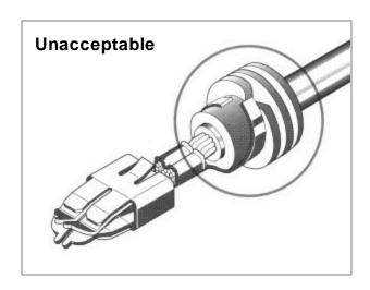
e) Also, check to be sure the crimp wings have not been over-crimped to the point of damaging the seal.
