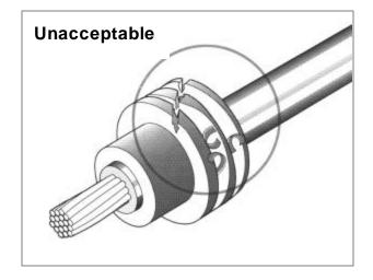
c) Check the outer edges or sealing surfaces of the seal to make sure that the seal itself is not damaged.
