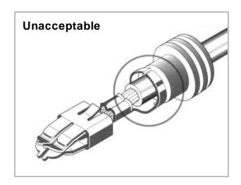
d) Check the crimp wings to be sure that the seal is well attached and secure, but not damaged in the sealing area itself.
