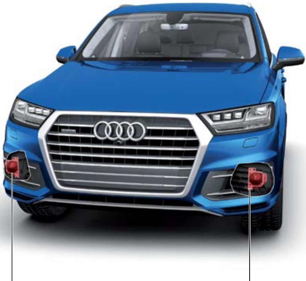
Right Adaptive Cruise Control Sensor and Distance Regulation Control Module J428 (master)
