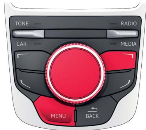
Button combination for system reset
