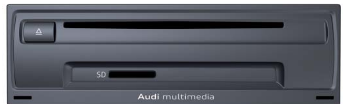
Front panel of J794 for Standard MIB, radio version
