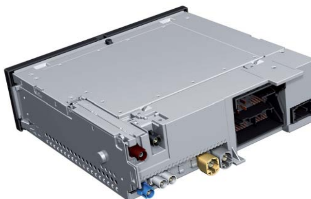
Rear panel of J794 for High-spec MIB with Audi connect inc. car phone
