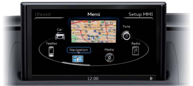
7.0" display for High-spec MIB on Audi A3 '13
