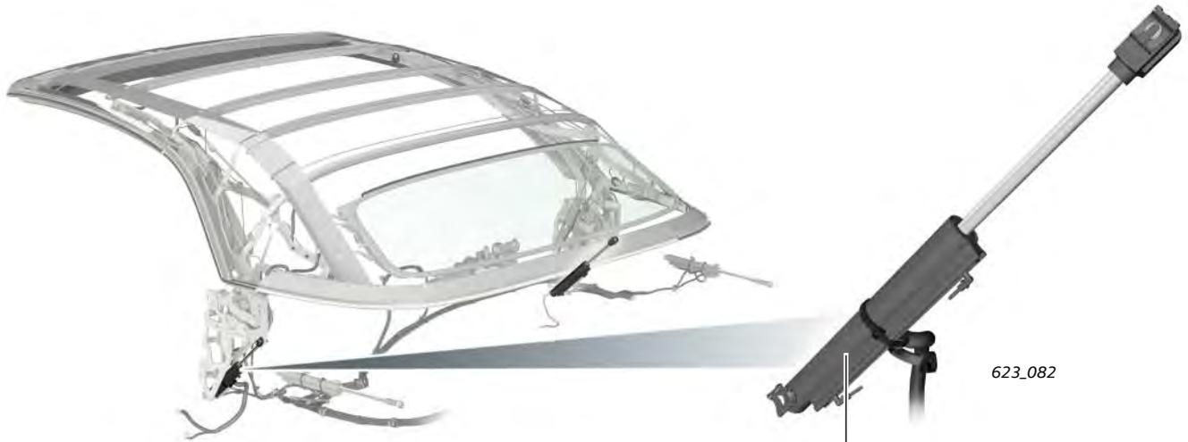
Hydraulic cylinder of main bearing
