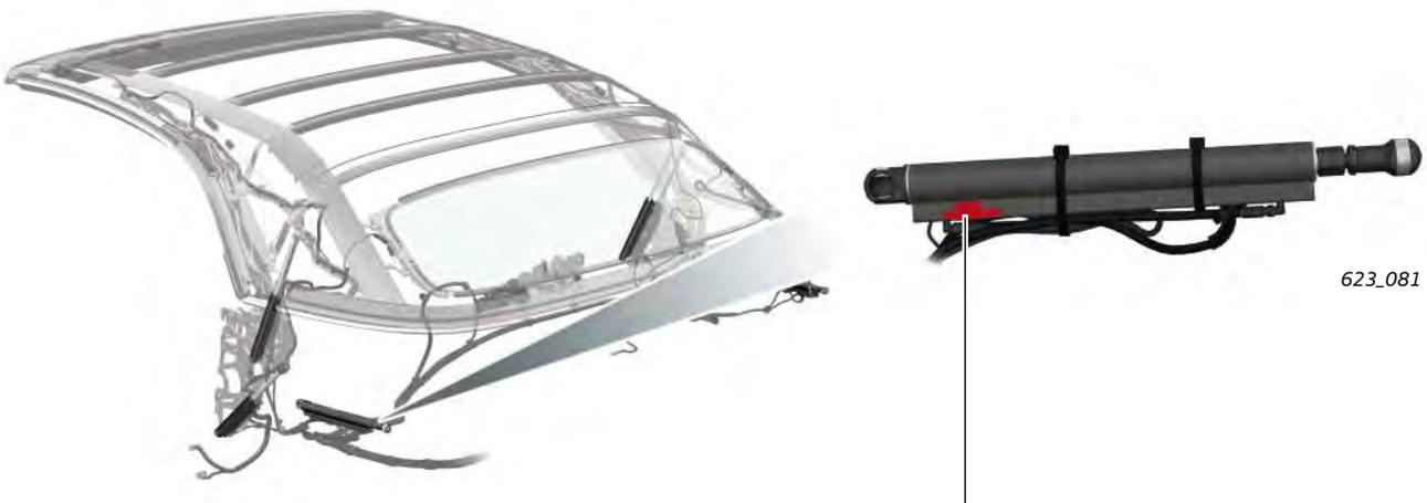
The convertible top box lid switch F407 is built into the cylinder
