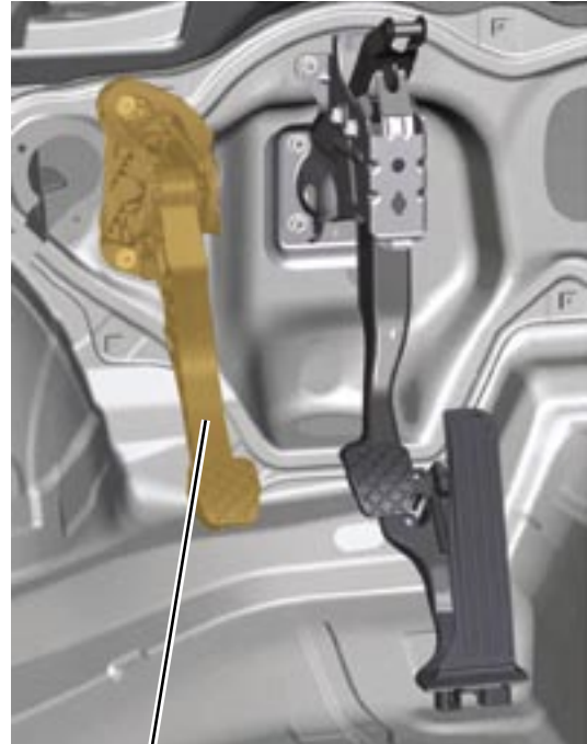
Clutch Pedal with Clutch Position Sensor
