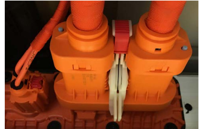
All HV wires in the ID.4 are connected mechanically. No screw connections on the wires are used.
