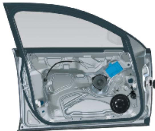
Installation position of door control module, driver side (01331) J386
