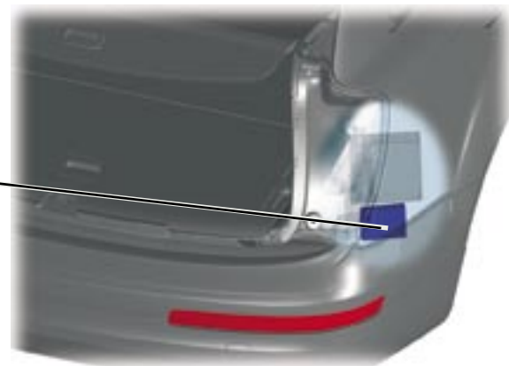
Installation location of the Keyless Access Authorization Antenna Reader J723
