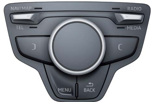
"Mid" control panel with manual gearbox
