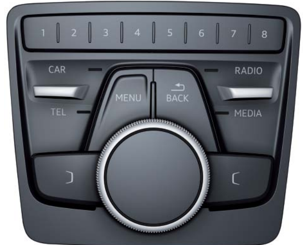
"Basic" control panel with automatic gearbox
