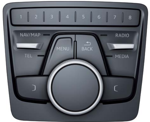
"Mid" control panel with automatic gearbox
