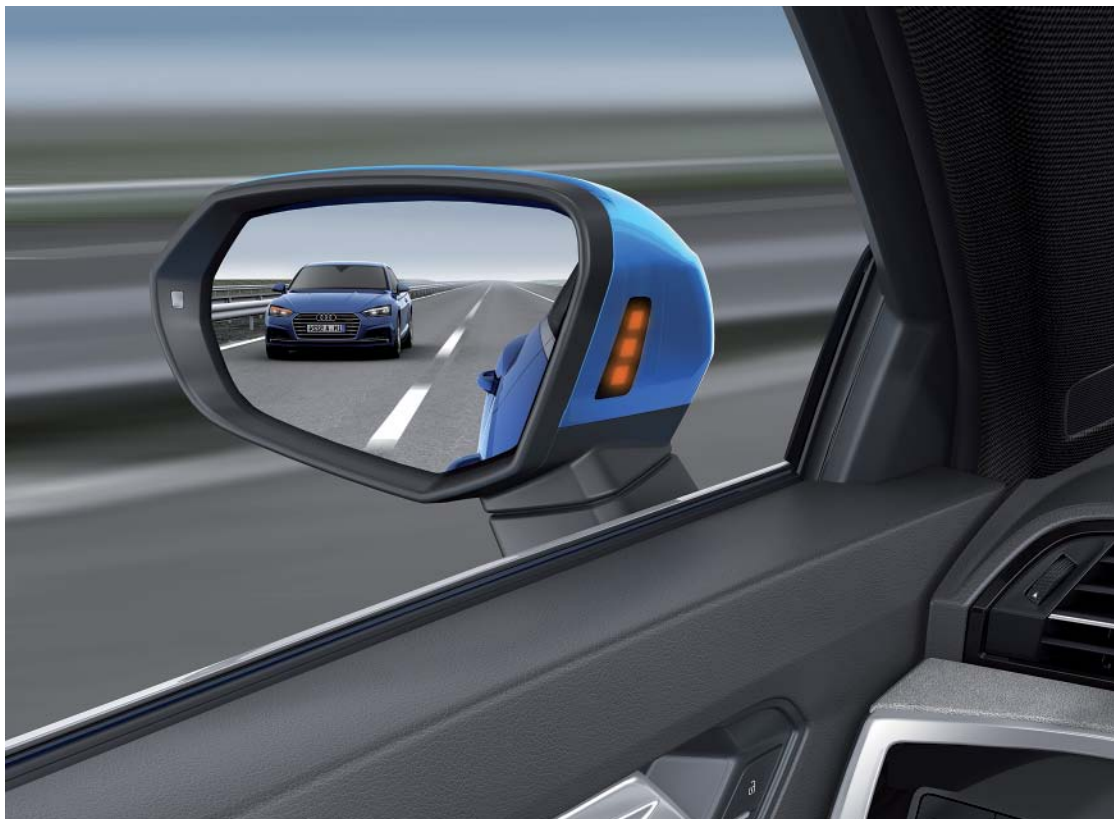
Active warning lamp for lane change warning in left exterior mirror
