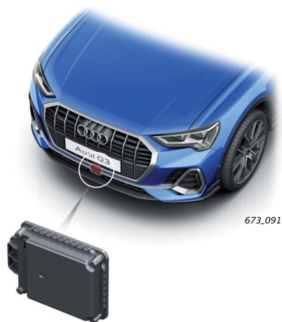
Right adaptive cruise control sender G259 and adaptive cruise control unit J428
